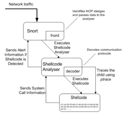
Figure 5 Shellcode analyser operation
